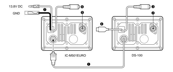
**NOTE:** Binding the GPS cable, GPS connector and clone receptacle with the water resistant tape, increases the water-proofing of the controller.
